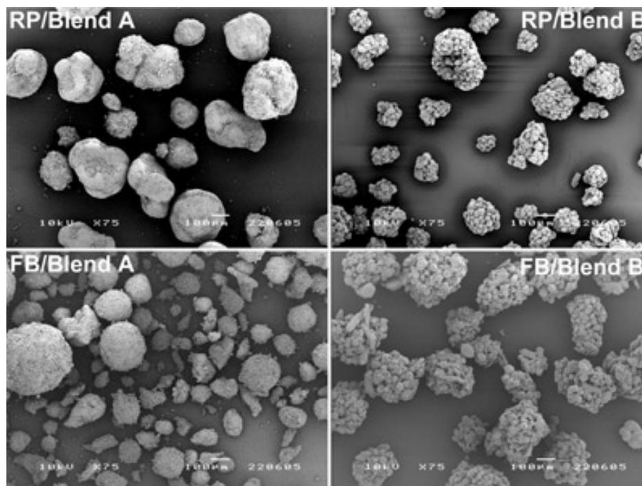
**Figure 4.** Scanning electron microscope pictures of granules from batches 2, 6, 10, and 14, all with low liquid addition and high fluidizing air flow rate. Magnification  $\times 500$ . RP indicates rotary processor; FB, fluid bed.
