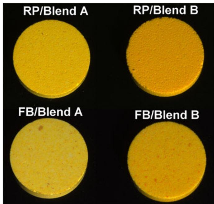
**Figure 5.** Digital images of tablets from batches 2, 6, 10, and 14, all with low liquid addition and high fluidizing air flow rate. RP indicates rotary processor; FB, fluid bed.
