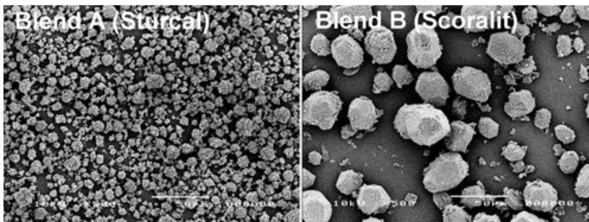
**Figure 1.** Scanning electron microscope pictures of the applied calcium carbonate grades Sturcal (Blend A) and Scoralit (Blend B). Magnification  $\times 500$ .
