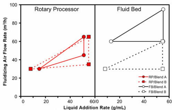
**Figure 2.** The determined working ranges of the RP and the FB. RP indicates rotary processor; FB, fluid bed.
