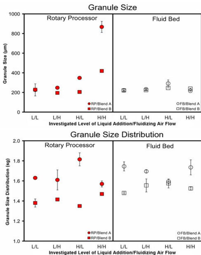
**Figure 3.** Effects of the investigated variables on granule size and granule size distribution. RP indicates rotary processor; FB, fluid bed; L, low; H, high. Error bars indicate the range of repeated experiments.
